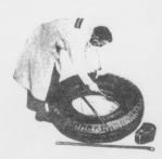
3. Lubricate last section of lower bead to facilitate mounting.
