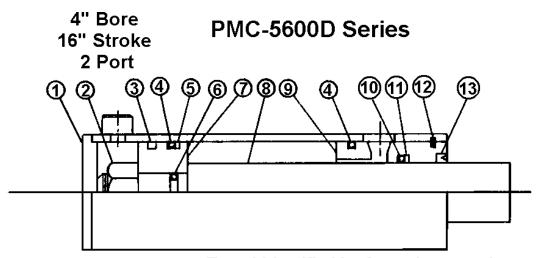
Type 4 identified by Snap ring securing gland cyl-pmc-5600d
