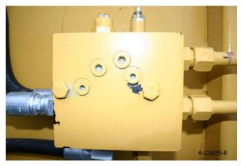
Visually there are several thing you can check to ensure you have the correct valve. The new valve (item #1) is 6" wide whereas the older valve (Item #3) was 5" wide. The new valve utilizes a unload cartridge that sticks outward on the side of the valve.
