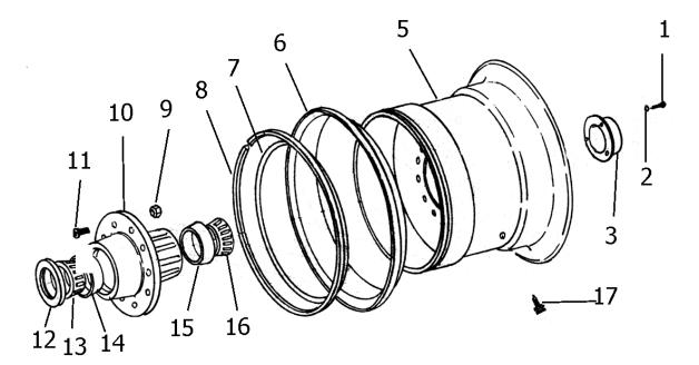
PARTS LIST FRONT WHEEL and HUB ASSEMBLY MODEL I-160 XL
