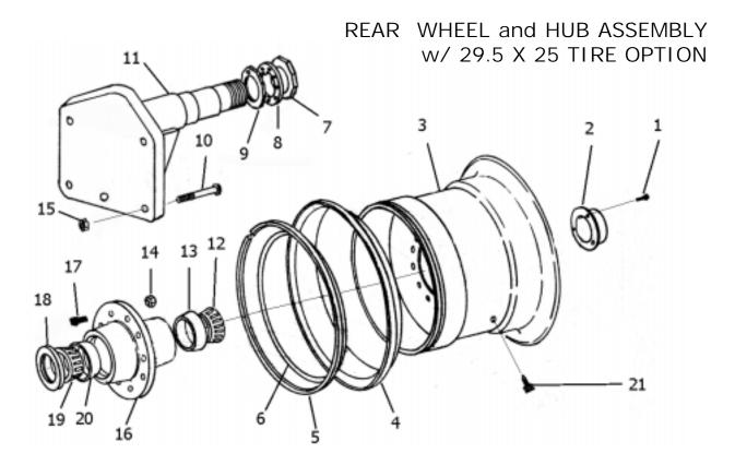
PARTS LIST REAR WHEEL and HUB ASSEMBLY - w/ 29.5 X 25 TIRE OPTION MODEL I-160 XL
