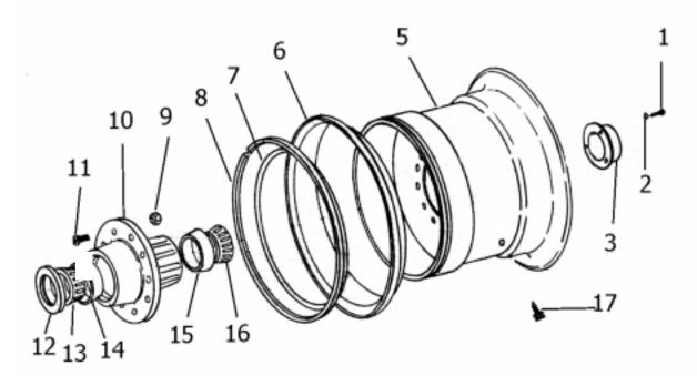
PARTS LIST FRONT WHEEL and HUB ASSEMBLY MODEL I-160 XL
