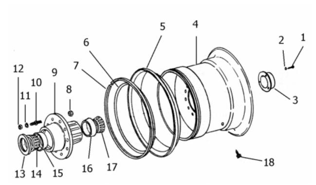
PARTS LIST FRONT WHEEL and HUB ASSEMBLY MODEL I-160
