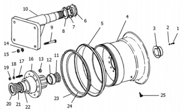
PARTS LIST REAR WHEEL and HUB ASSEMBLY MODEL I-160
