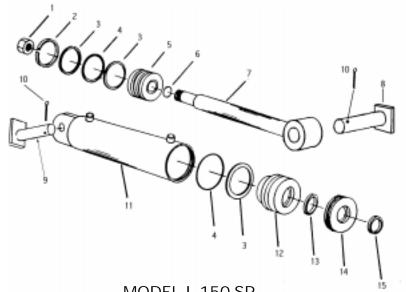
MODEL I-150 SP LIFT CYLINDER 5 X 20" PART NO. A520H275 (s.n. 20267 & above) 3/4" hyd ports PART NO. A520H200 (s.n. 20266 & below) 1/2" hyd ports serial number break occured on 6/8/00
