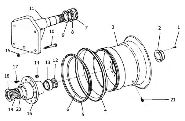
PARTS LIST REAR WHEEL and HUB ASSEMBLY MODEL I-150 SP
