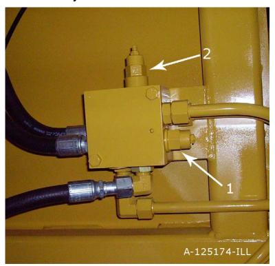
**IMPORTANT:** This Hyd. Manifold was integrated into production April, 2006 It replaces A125070 valve.
