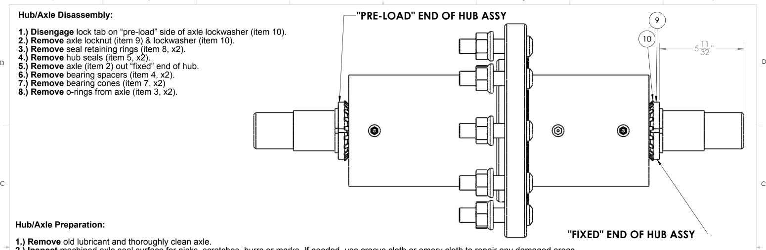
2.) Inspect machined axle seal surface for nicks, scratches, burrs or marks. If needed, use crocus cloth or emery cloth to repair any damaged areas.
