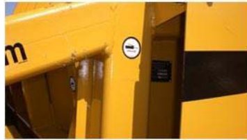
Grease Line - Rear
