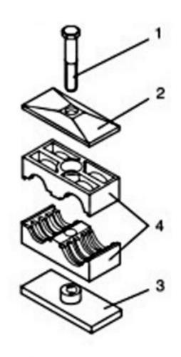
Twin Clamp with Weld Plate
