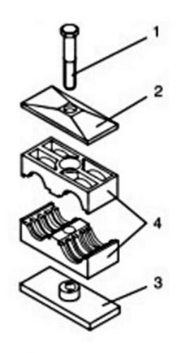
Twin Clamp with Weld Plate
