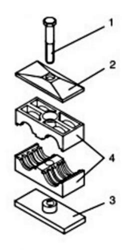
Twin Clamp with Weld Plate
