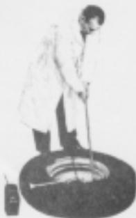
1. Remove valve core to deflate and loosen tire from bead seat on both sides. Lubricate upper bead of tire thoroughly. With stops toward rim, insert spoon ends of both tools about 10 inches apart. While standing on tire to hold bead in well, pull one tool back toward center of rim.
